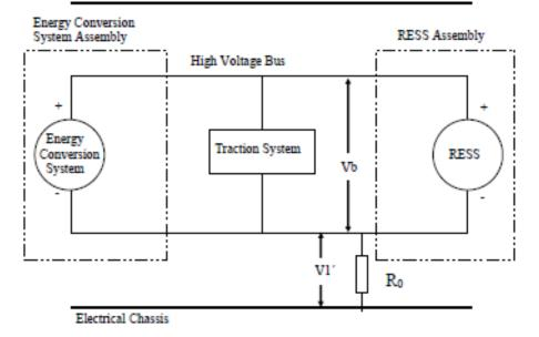
If V2 is greater than V1, insert a standard known resistance (Ro) between the positive side of the high voltage bus and the electrical chassis. With Ro installed, measure the voltage (V2') between the positive side of the high voltage bus and the electrical chassis. (See Figure 3). Calculate the electrical isolation (Ri) according to the formula shown. Divide this electrical isolation value (in ohms) by the nominal operating voltage of the high voltage bus (in volts).
