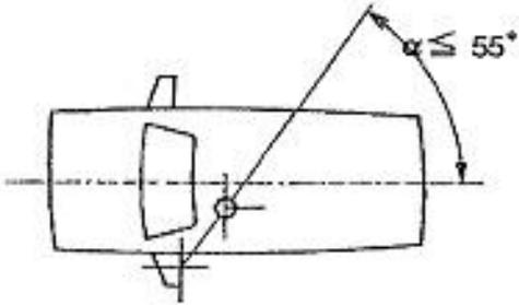
Figure 1: A vehicle showing the rear-view mirror and a line which joins the driver's two ocular points. The angle between the line of sight and the line to the mirror is  $\alpha \leq 55^\circ$ .
