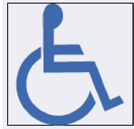
Figure : Identification marking for wheelchair accessible vehicle Size: at least 100 mm side, the ratio of length and width 1:1 Colour: white background with blue symbol
