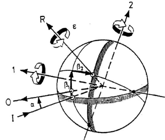
1: First Axis is fixed perpendicular to the plane containing the observation and illumination axis.
