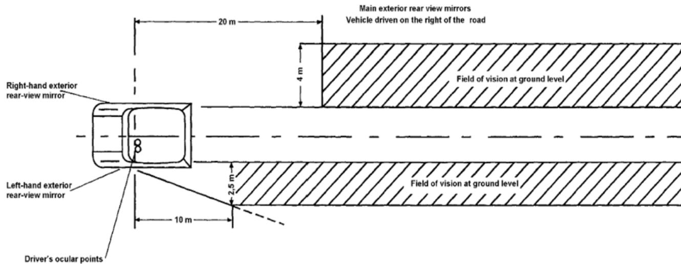
Figure 8: Field of vision of Class VII mirrors
