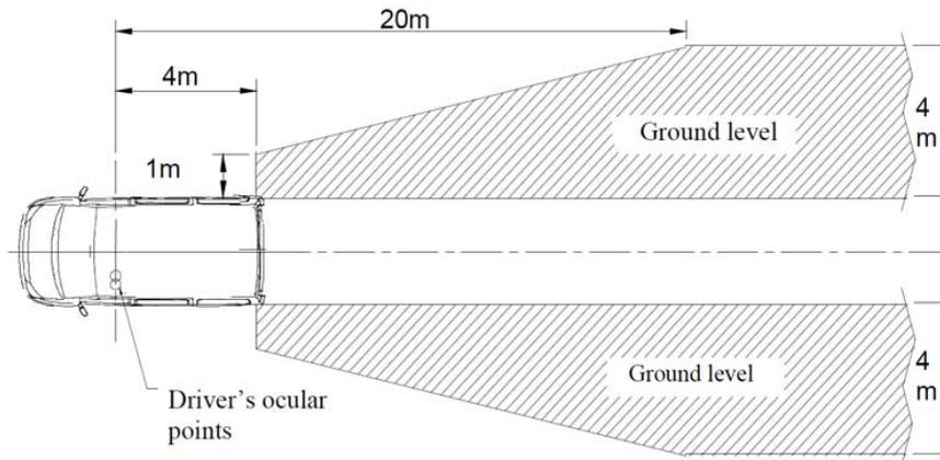
Figure 4: Field of vision of Class III mirrors
