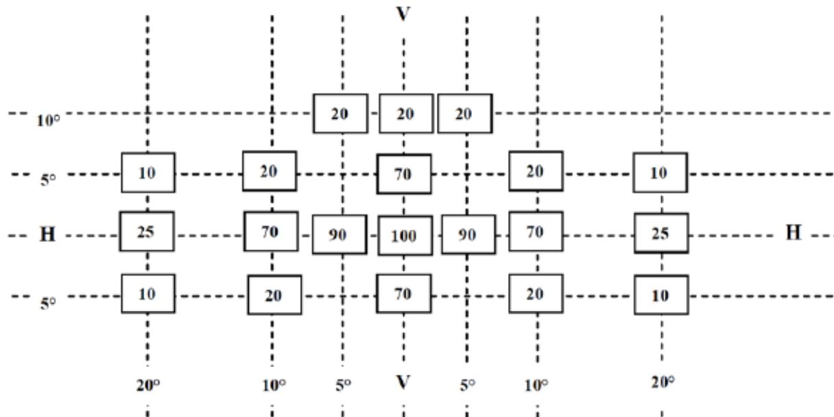
Figure 1: Table of standard light distribution
