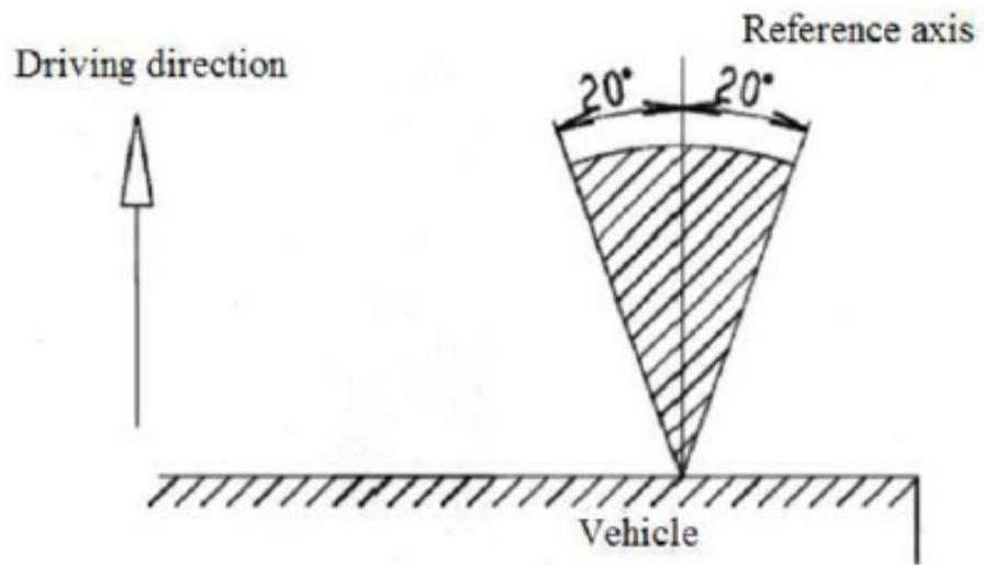
Figure 2: Minimum angles required for light distribution in space
