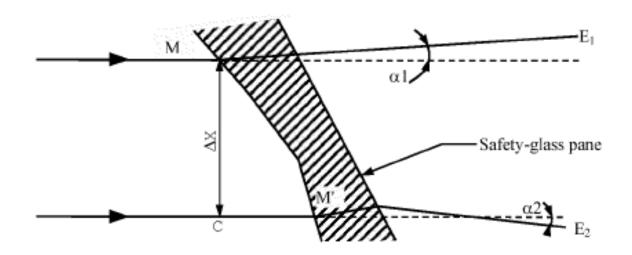
Note:  $\Delta \alpha = \alpha_1 - \alpha_2$  is the optical distortion in the direction M-M<sup>\*</sup>.
