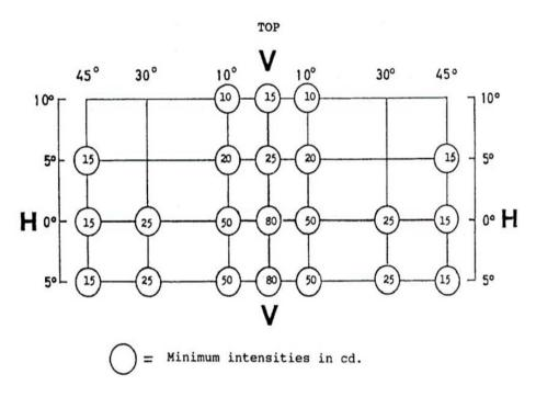
Table 1. Measuring points expressed in degrees of angle with the axis of reference and values of the minimum intensities (candelas) of the light emitted
